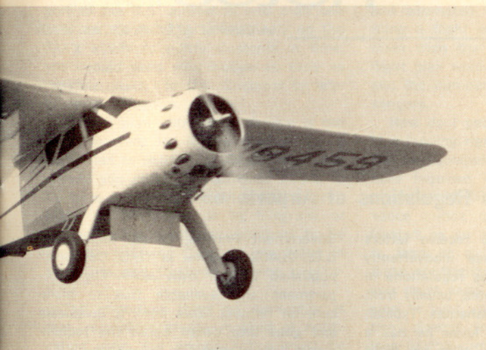
The C-38 was unique in having the flap under the belly. Note how the landing-gear legs have been bowed to widen the track. Photo by the author, 1964
